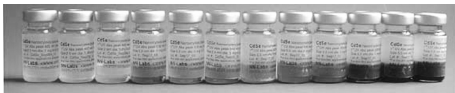
Fig. 2 : Fluorescence induced by exposure to ultraviolet light in vials containing various sized Cadmium selenide (CdSe) quantum dots (www.nn-labs.com)
